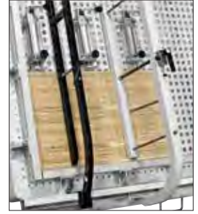
Fixed and sliding front clamp.
